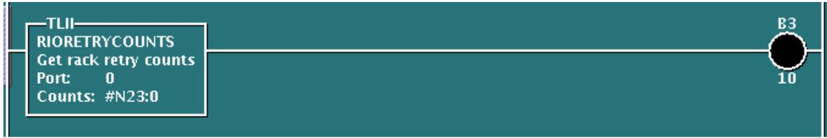
This permissive instruction is used to get the rack retry counter values (Counts) for a given RIO Interface (Port). Four words are allocated for each full rack where each word corresponds to the starting quarter rack offset (1st, 2nd, 3rd, and 4th). Thirty-two (32) racks are supported. Total length of the assigned file is 128 (4x32) words. Valid count range will be 0-255 (8 bits).
