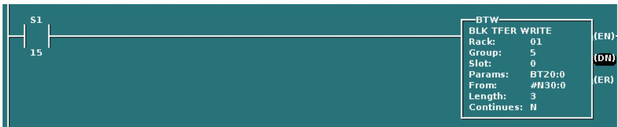
In this example, the BTW is executed one time during the first ladder scan to write configuration data to an analog Input Module.
