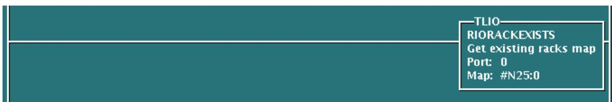
This output instruction creates a 32 word file (Map) of the existing racks on the specified RIO Interface (Port) network. Each word corresponds to a rack number where bits 8, 9, 10, 12 are set to indicate that adapters for 1st, 2nd, 3rd, or 4th logical quarter racks, respectively are present.
