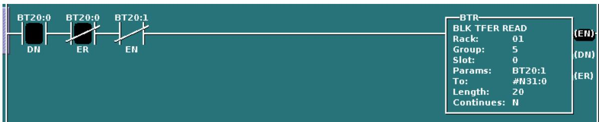
In this example, the BTR will be enable if the BTW was successful, assuring that the analog Input module was successfully configured. Then the BTR will be executed repeatedly during the ladder scan to read the analog input values.
