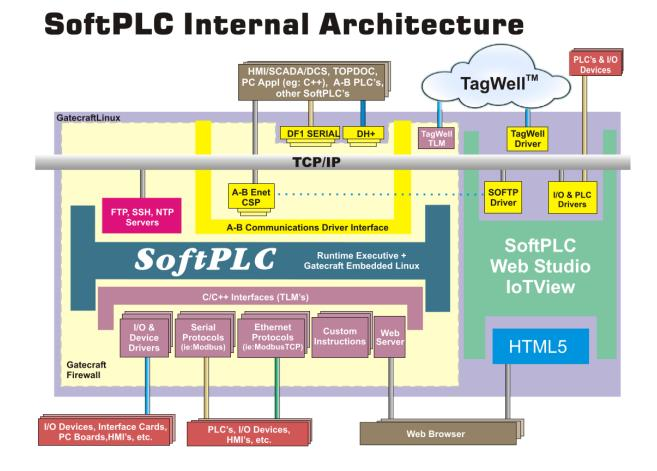
Most SoftPLC users require no knowledge of Linux - the operating system is transparent. Users interact with SoftPLC through TOPDOC NexGen software only (much like users of Rockwell Logix controllers have no knowledge/need to use the underlying O/S in those systems).
