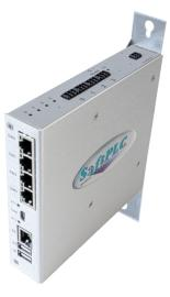
Any HMI/SCADA/DCS system can continue to be used, normally without change, as the SoftPLC will appear as an A-B PLC to the operator interface - either as a PLC-5/SLC-500 or using PLC-2 compatibility mode on serial DF1, DH+ or A-B Ethernet networks.
