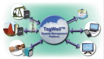
SoftPLC Gateways can provide access to other control systems via SoftPLC's TagWell Cloud Remote Management Platform, and via direct modem connections acting as a remote access switch and/or as a data concentrator.
