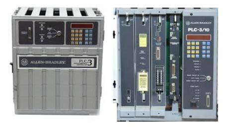
TOPDOC PLC-3 requires 32-bit WindowsXP or later\*. Communication to the PLC-3 can be direct to the programming port through a null modem serial cable or over DH/DH+ with a 1784-PKTx/KTx interface card or external interface such as a 1770-KF2B. The 1784-PCMK is not supported.
