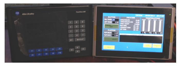
By "drop-in" we mean that the Web Studio HMI will fit into the existing panel cut-out. In almost all cases, the Web Studio HMI is slightly larger than the PanelView, so no coverplate would be required, just minor filing/cutting. Where the Web Studio HMI is smaller than the PanelView, the difference is usually minor.
