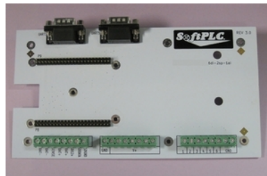
I/O Board (Cat No SPBB-6DI2SP1AI) provides (2) RS-232 and an SDI-12 interface for Micro Gateway models SPBB-x
