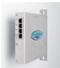
Smart SoftPLC w/ no local I/O interface + optional bracket (most popular A-B Migration configuration)
