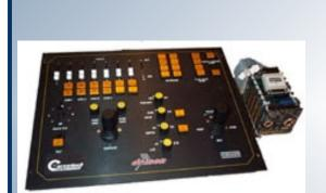
"On the surface ship, a control panel of switches and joysticks connected directly to a SoftPLC communicate with a network of 1 or more subsea SoftPLC controllers up to 5km away through fiber optic links bringing video, telemetry, Ethernet and analog or digital sonar data back to the operators. Fast, efficient and highly robust.
