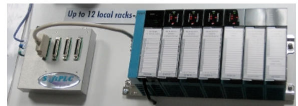
Smart SoftPLC connected to I/O Rack via I/O Expansion Cable
