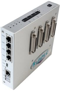
**Huge Local I/O Capacity:** A Smart SoftPLC can support up to 12 local racks - at 256 points per rack that means up to 3072 points of fast update local I/O!
