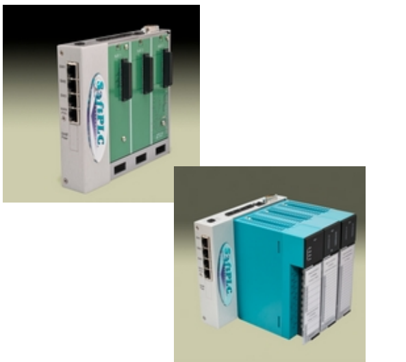
Figure 2.14: Remote Drop with Backplane3
